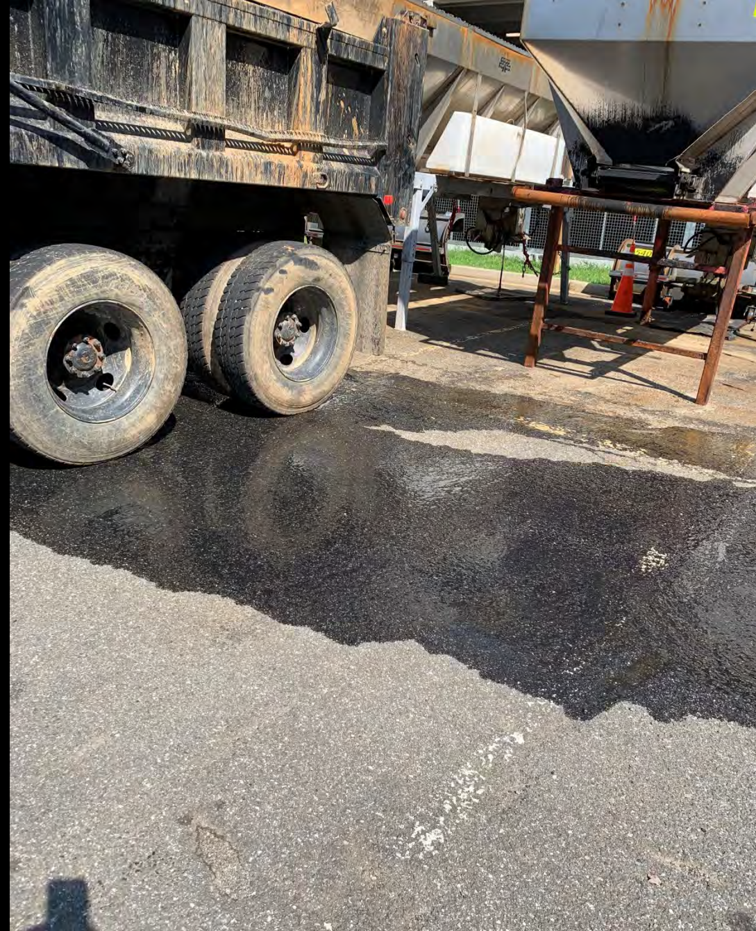
Leak of hydraulic fluid from dump truck
