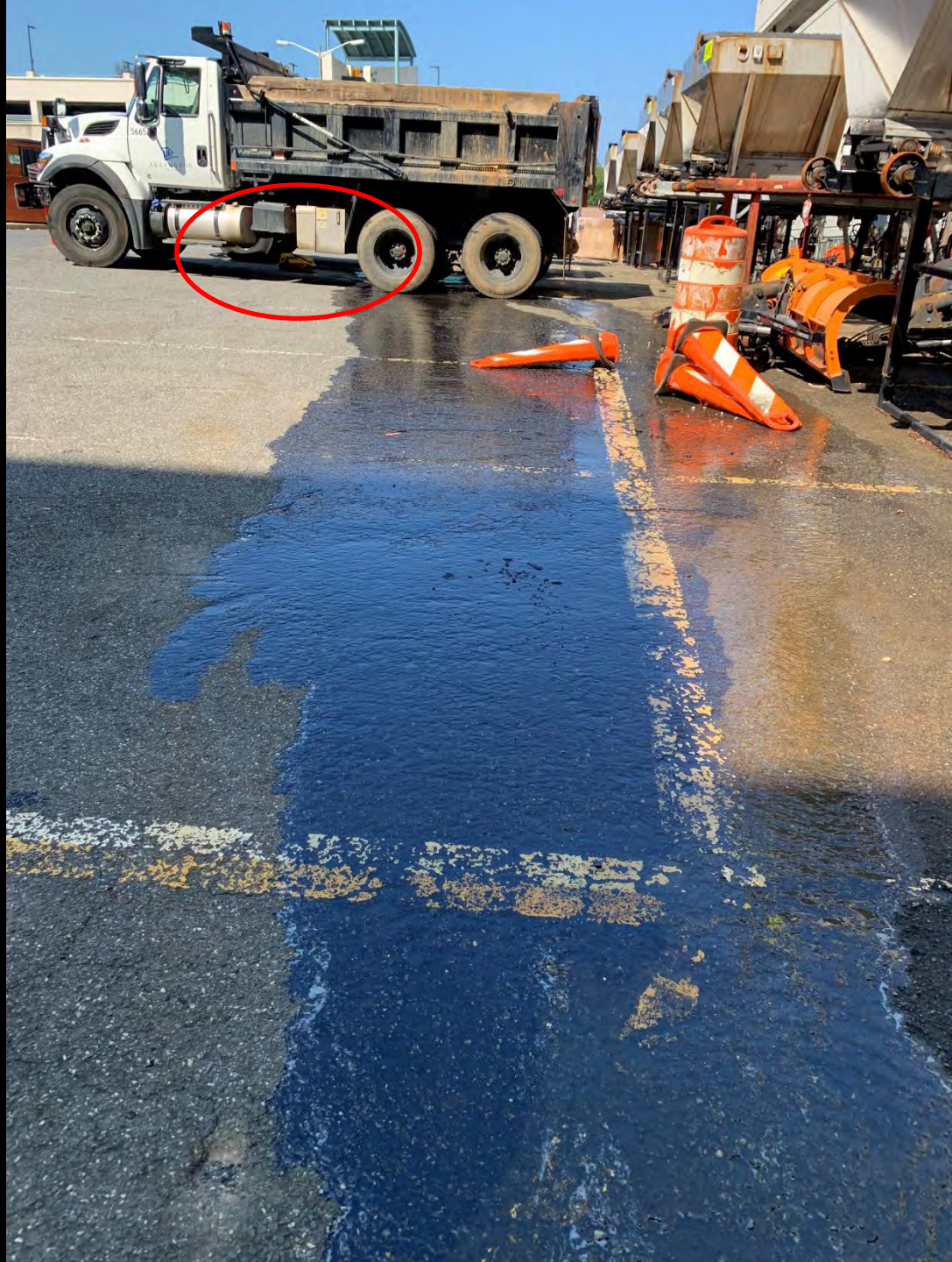
Leak of hydraulic fluid from dump truck
