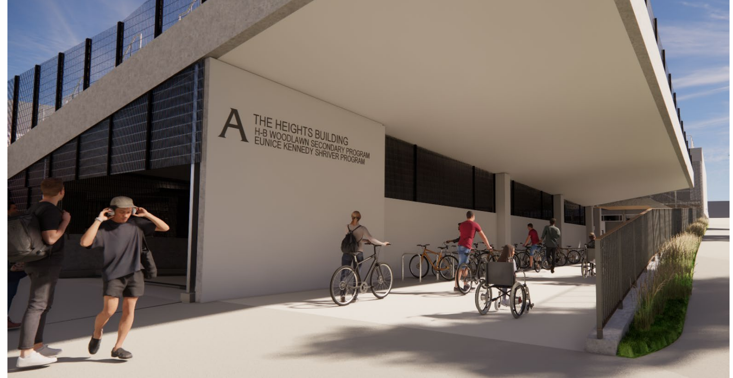
Proposal: a high-quality white mineral coating applied to the concrete wall and soffit at covered entrance.
