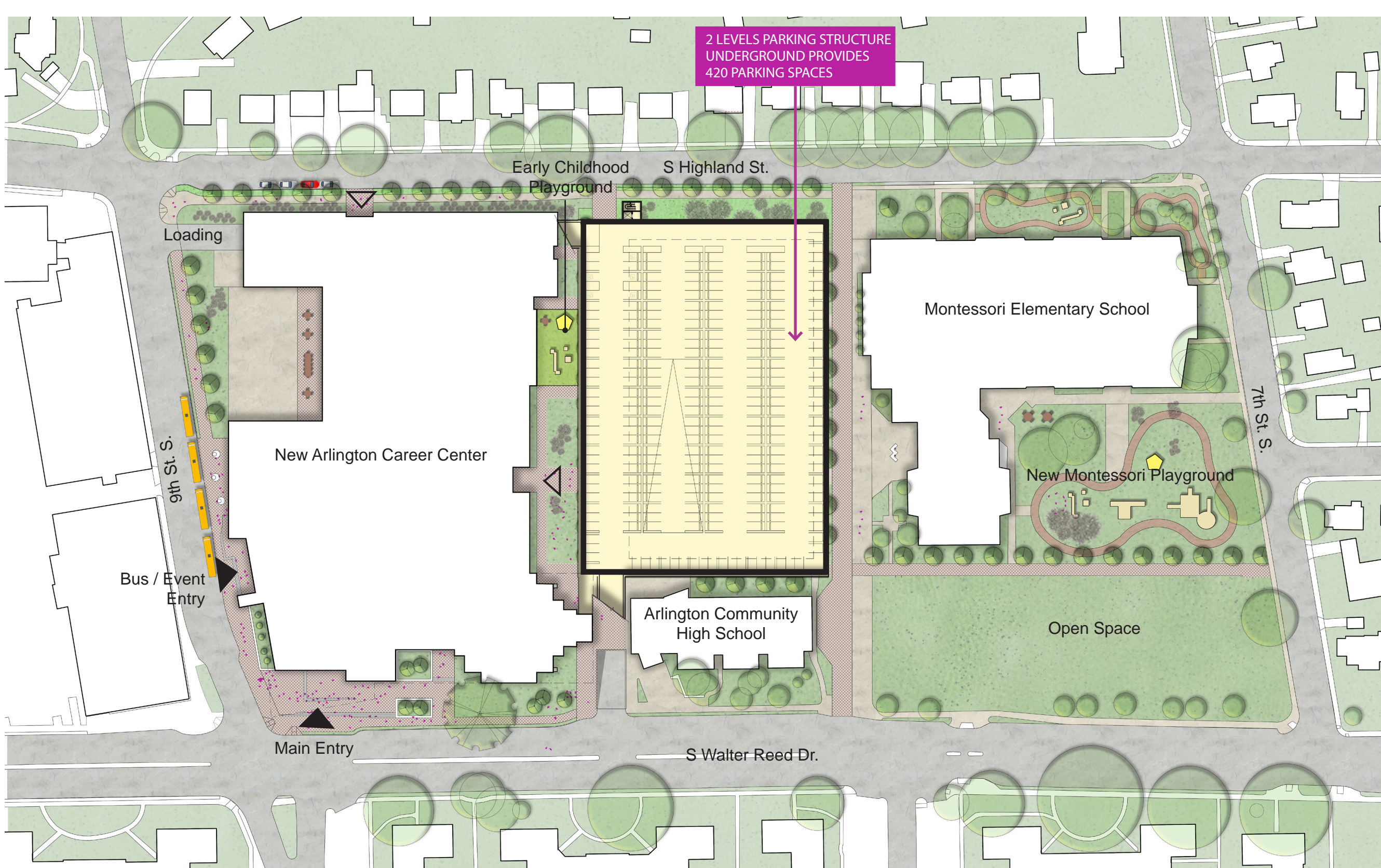
Parking Option 1 (Two Levels Underground)
