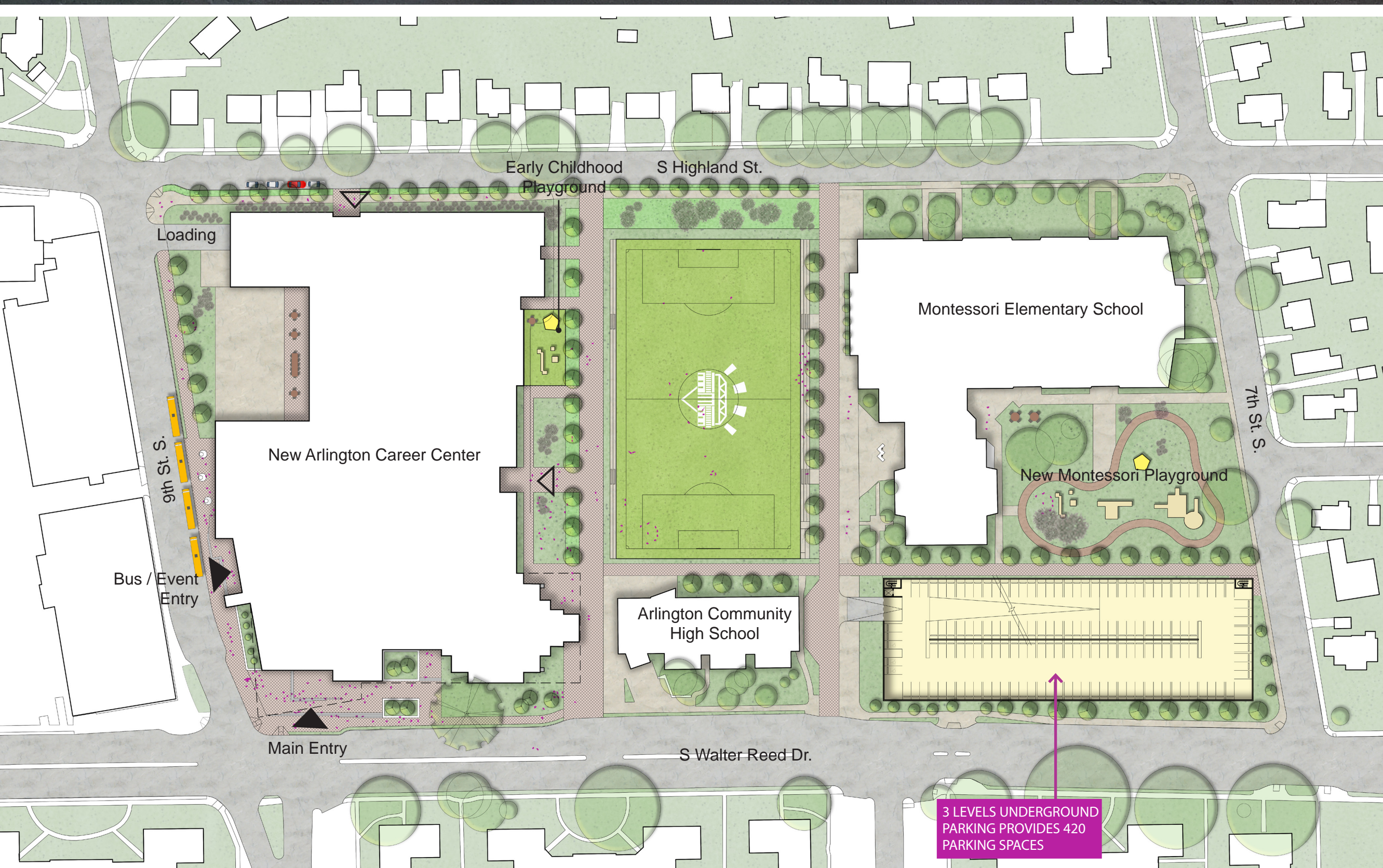
Parking Option 3 (Three Levels Underground)
