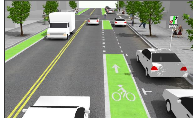
Enhanced markings (green paint)
